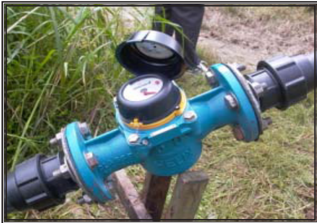
Water meter installed at flower under rain shelter plot at Sg Telom
