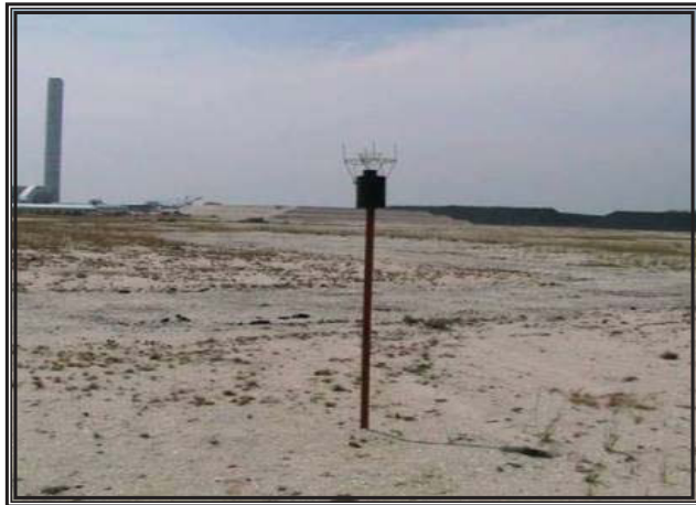
One of the 10 dust deposit gauges installed at TNBJ
