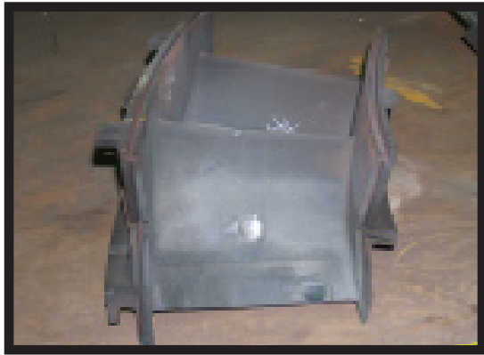
First stage nozzle premature failure
