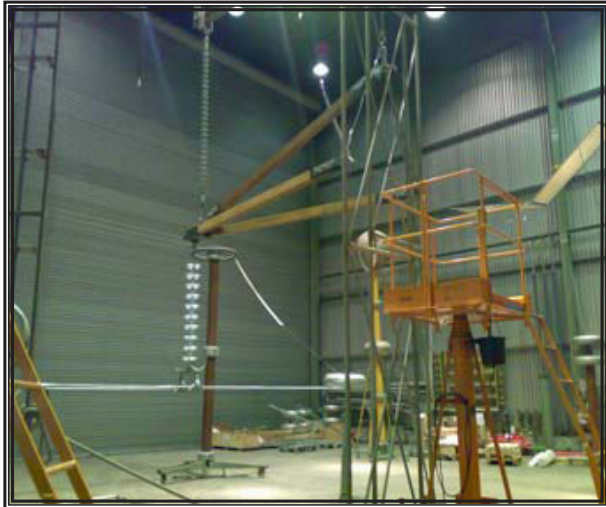
Electrical Testing of Cross Arm
